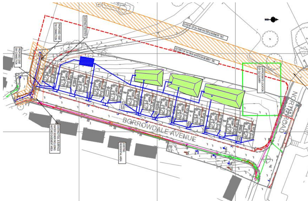
Figure One – Proposed Surface Water Drainage Scheme
